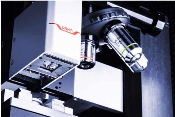
Figure 6: The UNHT 3 ultra-nanoindentation device with the patented surface referencing.
